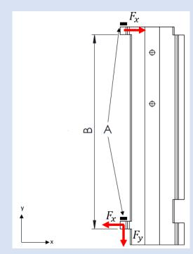
A locking mechanism must be implemented at the hinges, marked A, to secure the module from vertical displacement.
