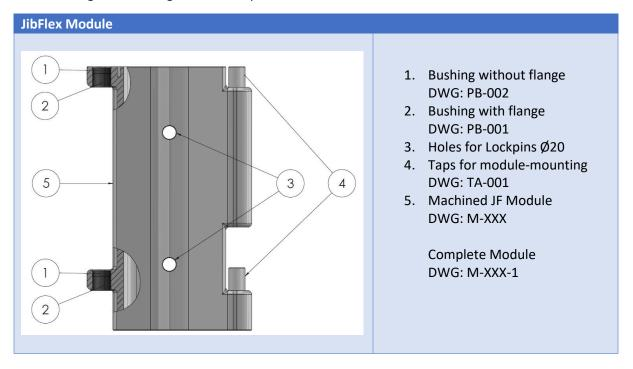
The modules are designed such that a rotation of 62° can occur between one module and the previous. This yields a turning diameter of approximately 500 mm as illustrated below:
