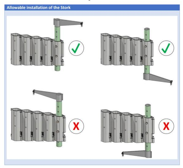
The Stork must be placed in the last module as shown above. The procedure for a general stork is shown on the following illustrations.
