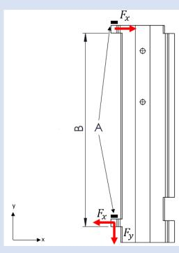
A locking mechanism must be implemented at the hinges, marked A, to secure the module from vertical displacement.
