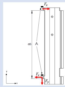
A locking mechanism must be implemented at the hinges, marked A, to secure the module from vertical displacement.
