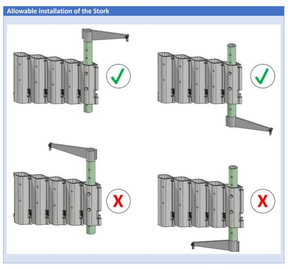
The Stork must be placed in the last module as shown above. The procedure for a general stork is shown on the following illustrations.
